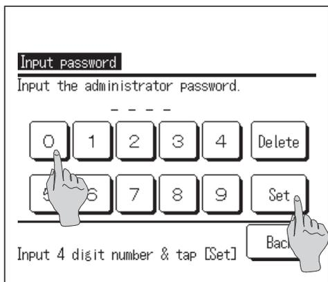
6 When an item is referenced to the administrator password in this manual, the Input password screen is displayed after selecting the menu.
