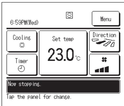
When one IU is controlled with 2 R/Cs, the following settings cannot be made on the sub R/C. It is necessary to use the main R/C. In case of the sub R/C, the icon **S** is displayed on the R/C screen.
