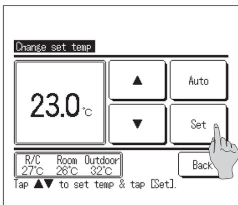
5 When the **Set** button is displayed on the setting screen for each item, tapping this button to confirm the setting.
