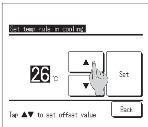
**8** Set the indoor temperature to start operation in cooling after setting the “Determine temp rule in cooling”.
