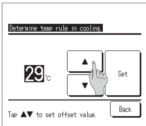
**6** Set the outdoor temperature for the “Determine temp rule in cooling”.
