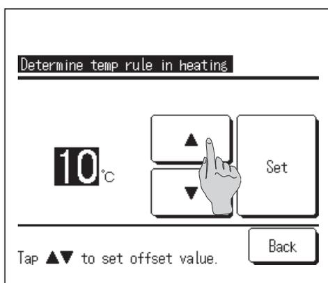
**7** Set the outdoor temperature for the “Determine temp rule in heating”.
