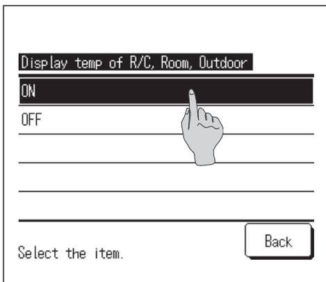
**9** Select ON/OFF for the display of the R/C sensor temperature, room temperature and outdoor temperature.
