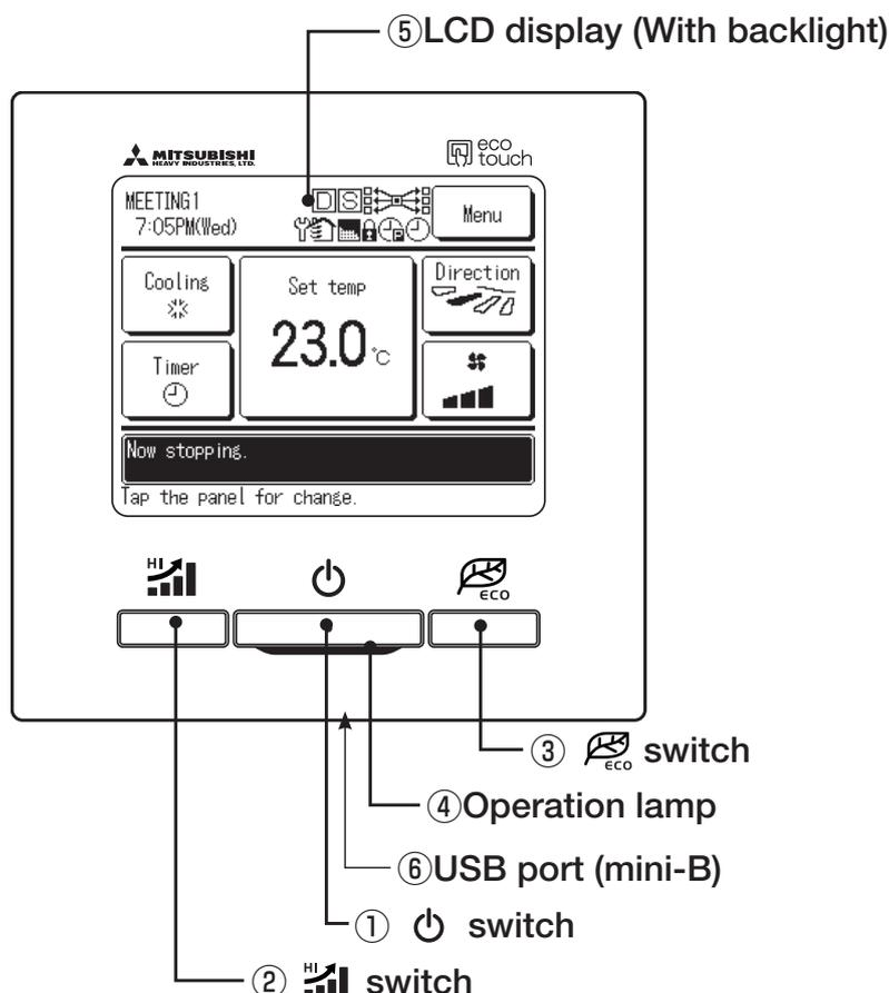
Touch panel system, which is operated by tapping the LCD screen with a finger, is employed for any operations other than the ① Run/Stop, ② High power and ③ Energy-saving switches.
