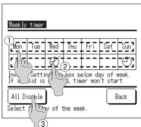
**5** When a desired day of the week ① is tapped on the display, contents of current setting for the day are displayed. (☞ 7)
