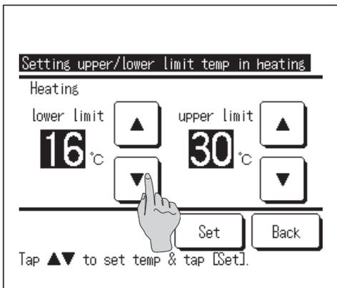
**1** When the “Setting temp range” is tapped on the administrator settings menu screen, the setting temp range menu screen is displayed.
