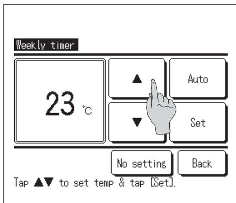
**11** Select a desired temperature (at 1°C intervals) with the ▲ ▼ buttons. Or tap the Auto button to select the Auto temp setting.
