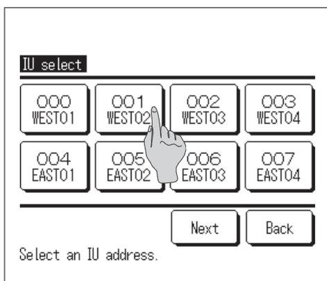
**3** When two or more IUs are connected to one R/C, an IU list is displayed. Tap the IU No. to be set.
