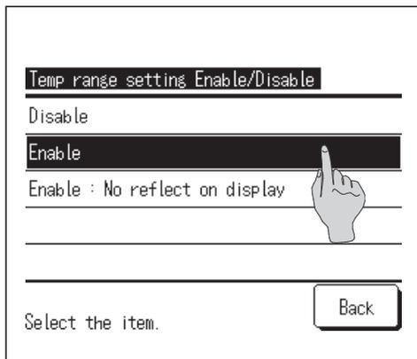
**4** Select the control contents of restriction on the setting temperature range.
