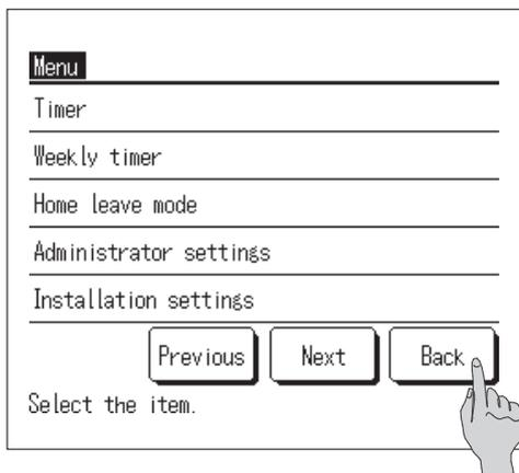
4 When the **Back** button is tapped, the display returns to the TOP screen.
