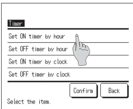
1 Tap the **Timer** button on the TOP screen or tap the **Menu** button on the TOP screen, and select the “Timer” on the main menu screen.
