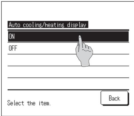
**8** Select ON/OFF for the display of the Auto cooling or heating.
