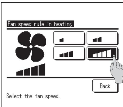
**11** Set the fan speed in heating mode.
