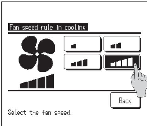
**10** Set the fan speed in cooling mode.
