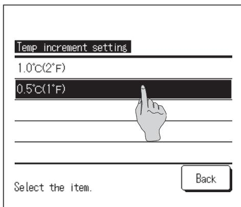
**1** When the “Temp increment setting” is tapped on the administrator setting menu screen, the Temp increment setting screen is displayed. Tap a desired temperature increment.
