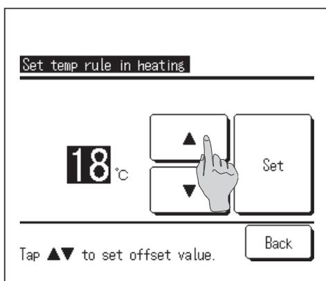
**9** Set the indoor temperature to strat operation in heating after setting the “Determine temp rule in heating”.
