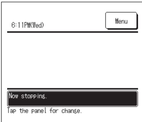
When the operation stops, all operation buttons on the screen turn off. When the set lighting time of backlight (
