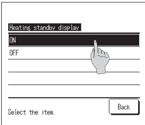
**6** Select ON/OFF for the Heating standby display.
