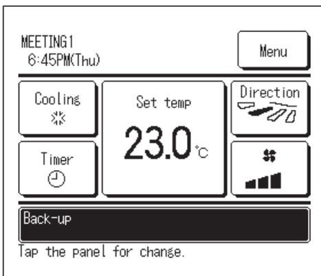
When the "Back-up" is displayed, contact your dealer immediately for checking.
