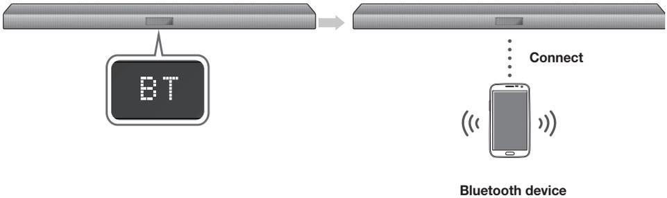
1. Press the
