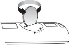
1. Use a suitable coin to turn the remote control's battery cover counterclockwise to remove it as shown in the figure above.
