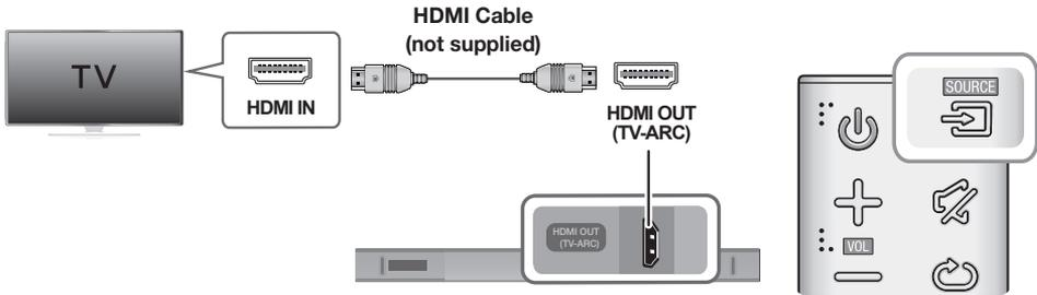
1. Connect an HDMI cable (not supplied) from the **HDMI OUT (TV-ARC)** jack on the bottom of the product to the HDMI IN jack on your TV.
