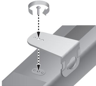
6. Use the two **Screws** (M4 x L14) to attach both **Bracket-Wall Mount L** and **R** to the Soundbar's bottom. For a proper fit, make sure to align the bumps on the Soundbar to the holes on the brackets.
