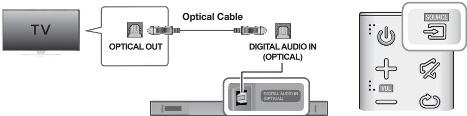
1. Connect the **DIGITAL AUDIO IN (OPTICAL)** jack on the Soundbar to the **OPTICAL OUT** jack of the TV with a digital optical cable.
