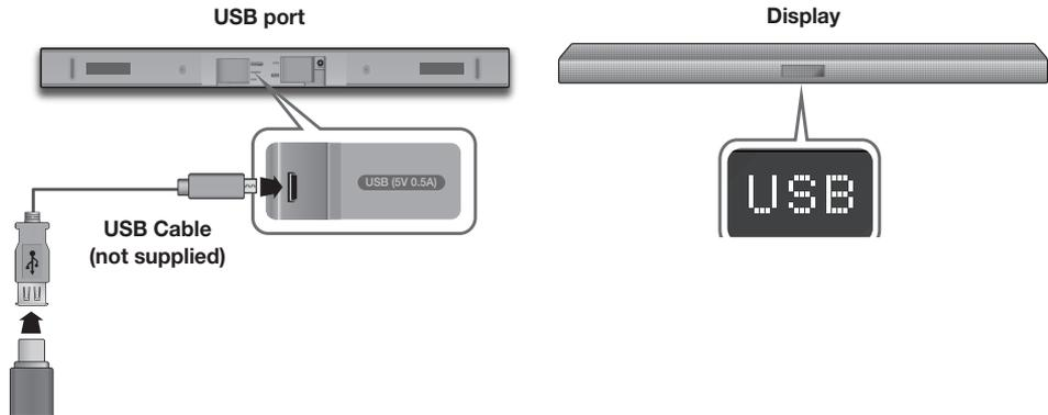
1. Connect a USB adapter cable with a male USB 2.0 Micro USB plug (Type B) on one end and a standard female 2.0 USB jack (Type A) on the other end to the micro USB jack on your Soundbar.
