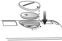
2. Insert a 3V lithium battery. Keep the positive (+) pole facing up when inserting the battery. Put the battery cover on and align the '•' marks side by side as shown in the figure above.
