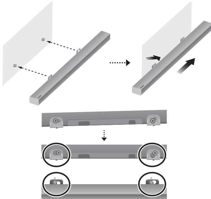
7. Install the Soundbar with the attached **Bracket-Wall Mounts** by hanging the **Bracket-Wall Mounts** on the **Holder-Screws** on the wall.
