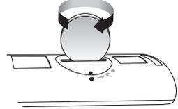
3. Use a suitable coin to turn the remote control battery cover clockwise as far as it will go to fix it in place.
